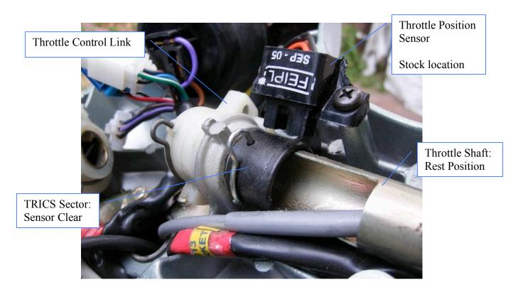
TRICS sensor is unblocked at rest to half throttle.
