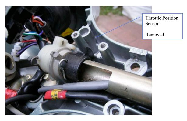
Unscrew two screws and rotate the sensor 180 degrees.
